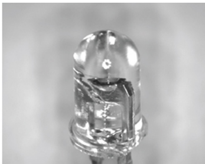
AM4115FKT (The infrared light penetrates LED)
